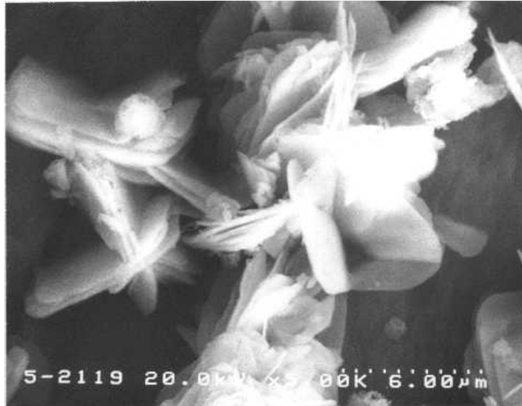
FIGURE 5. Examination of a uranium-rich area on an apatite grain from the high ionic strength column
